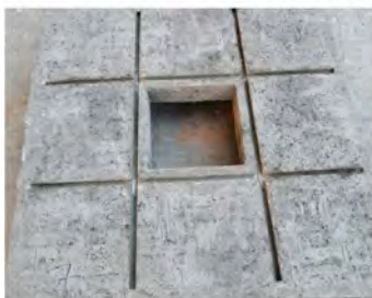
Slab strengthening by NSM technique with a GFRP rod along the edges of the opening.
