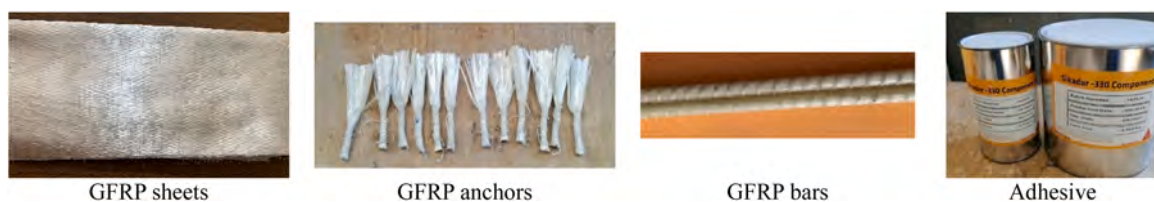
Fig. 3. Materials used for strengthening in this study.
