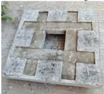
Slab strengthening by NSM technique by adding a layer of concrete.
