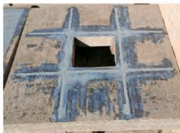
Slab strengthening by NSM technique with a GFRP rod along the edges of the opening.
