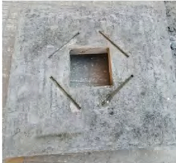
Slab strengthening by EBR technique with rods at the corners of the opening.
